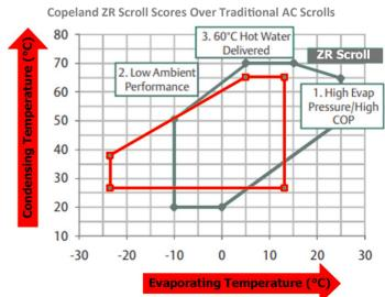
or To Operate At Low Ambient & Higher Condensing Temperature Vs AC Compressors
